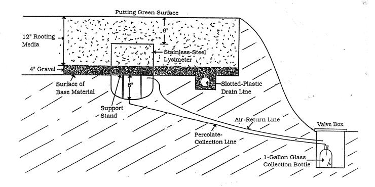
Fig. 8. Schematic of the free-draining stainless-steel lysimeter installation used in three greens at the Breakers West Golf Course in Palm Beach County, Florida.
